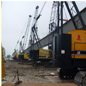
Cranes with replaced engines perform to cleaner emission standards.
